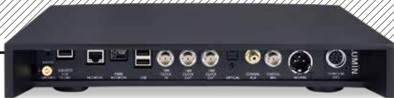
ABOVE: This 'Ethernet bridge' has RJ45 and SFP inputs, two USB-A ports for external drives alongside an isolated USB-B port (768kHz/DSD512) and S/PDIF outputs on coax, BNC, AES/EBU and optical (192kHz/24-bit). Note the trio of 10MHz clock ports
