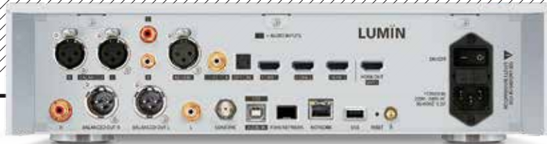
ABOVE: Busier on the back, the P1 offers analogue ins on XLR/RCA with digital ins on coax, optical and AES/EBU [all 192kHz/24-bit; DoP64], USB-B and optical/wired Ethernet ports [384kHz/32-bit; DSD512]. Three HDMI ins/one out, an S/PDIF (BNC) out and USB-A output are joined by fixed/variable preamp outputs on XLR/RCA
